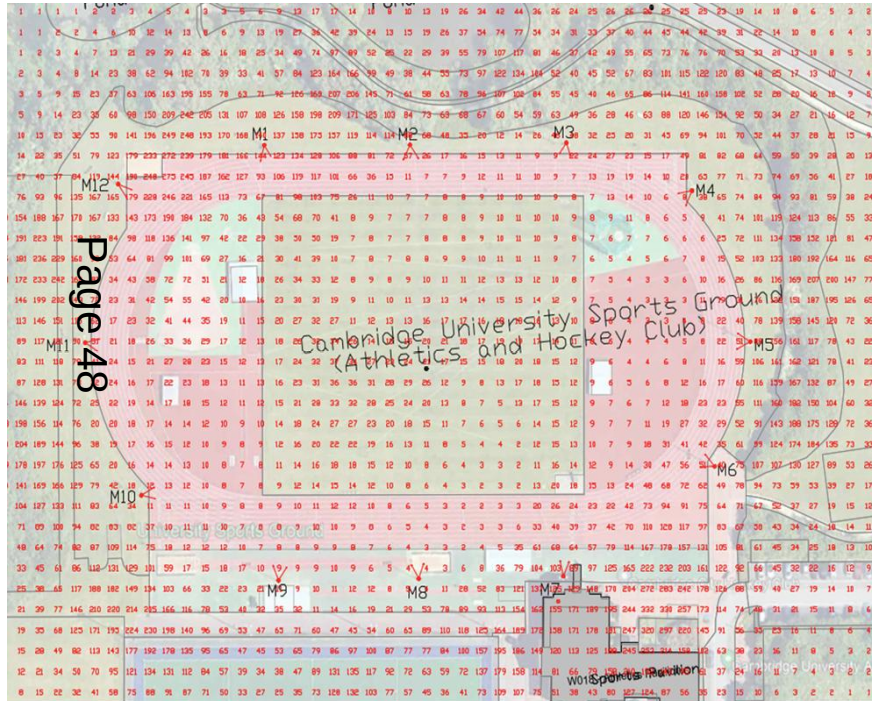
Figure 3: Existing Floodlighting Vertical Spill
